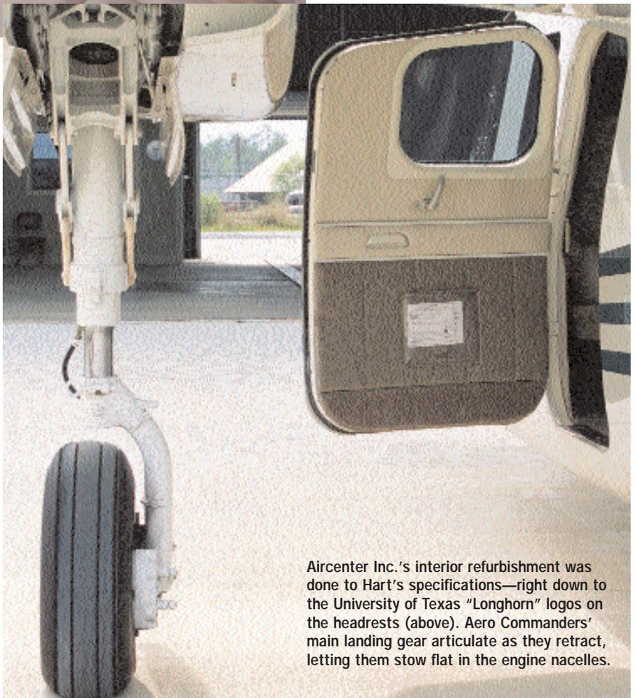
Aircenter Inc.'s interior refurbishment was done to Hart's specifications—right down to the University of Texas "Longhorn" logos on the headrests (above). Aero Commanders' main landing gear articulate as they retract, letting them stow flat in the engine nacelles.
